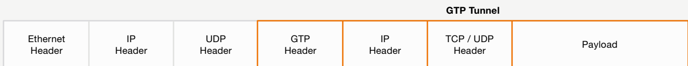
FIGURE 6 GTP tunnel frame format
