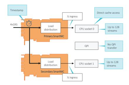
Relying on the QuickPath Interconnect (QPI) for distribution would diminish performance and impair scalability. To avoid this, the socket load balancing feature distributed the traffic between a primary and secondary SmartNIC and created a dedicated packet stream to each of the two CPU sockets, hereby bypassing the QPI.
